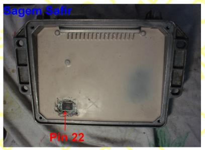
After cutting off the immo cable from the plug of Engine Control Module, by head of the cable connect pin 22 of flash 28F512, connect supply plug to the car cigarette lighter and turn on the ignition. Wait one minute till LED emulator will turn off.
