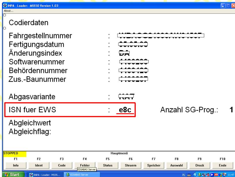
**Read code ISN from Engine Control Module or
